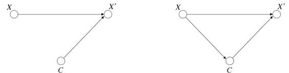
(a) Open-loop control. (b) Closed-loop control.
