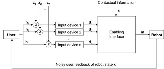
Fig. 1. Simplified representation of the complete human-machine system.
